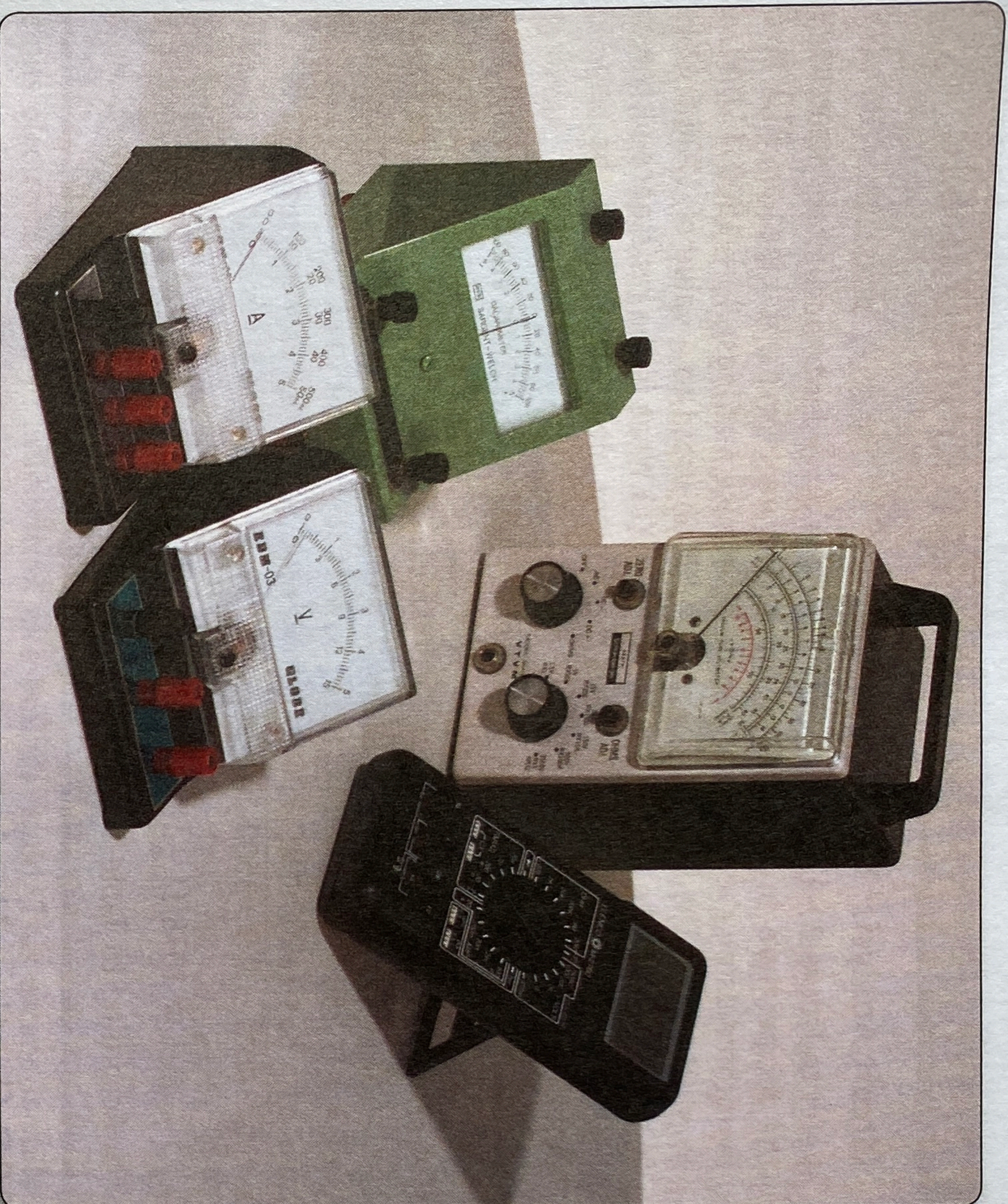
20-26 An ammeter, a voltmeter, and a galvanometer, the analog and digital multimeters (in back and right) can act as an ohmmeter as well as an ammeter and a voltmeter.
