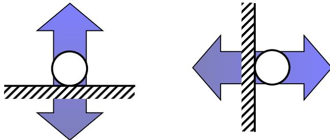
A **roller** support can support a structure in only one dimension.
