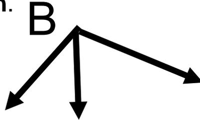
**As forces are solved, update free body diagrams.** Use correct magnitude and sense for subsequent joint free body diagrams.
