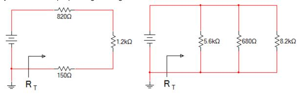
3. Using the laws of circuit theory, solve for  $R_T$ ,  $I_T$ ,  $V_1$ ,  $V_2$ , and  $V_3$ . Be sure to put your answer in proper engineering notation and use the correct units.
