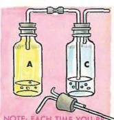
NOTE: EACH TIME YOU MOVE THE GAS-COLLECT-ING BOTTLE B FOR EXPERI-MENT, CONNECT BOTTLES A AND C TO PREVENT CHLORINE FROM GETTING OUT IN THE ROOM.
