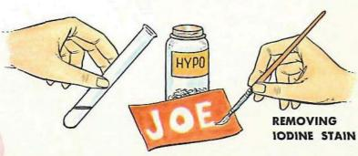
PAINT PAPER WITH IODINE. DISSOLVE A FEW CRYSTALS OF SODIUM THIOSULFATE ("HYPO") IN WATER. PAINT WITH THIS SOLUTION OVER THE BROWN COLOR. YOU WILL GET WHITE LETTERS AS HYPO FORMS COLORLESS COMPOUND WITH IODINE.
